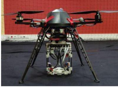
**FIGURE 15.18** The drone-embedded microphone array system used for creating the DREGON dataset (Strauss et al., 2018; Deleforge et al., 2019; IEEE Signal Processing Cup Syllabus, 2019).
